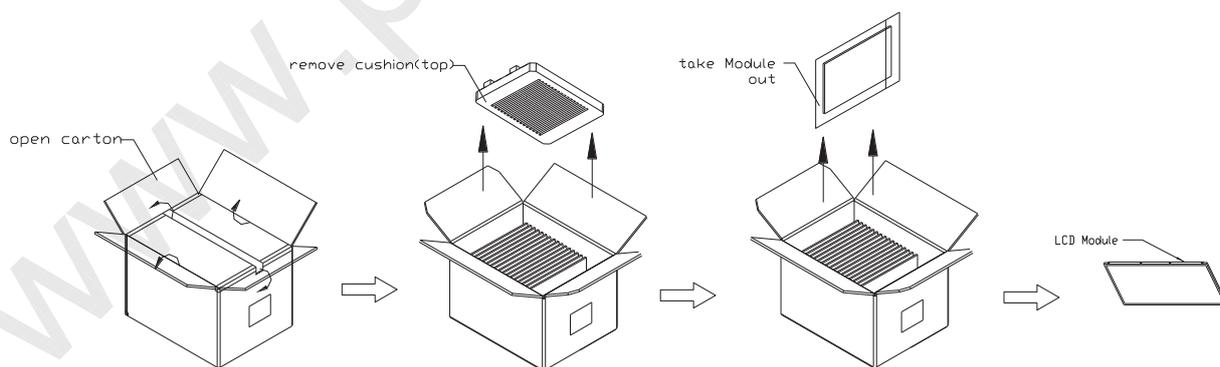
Figure. 9-3 UN-Packing method
