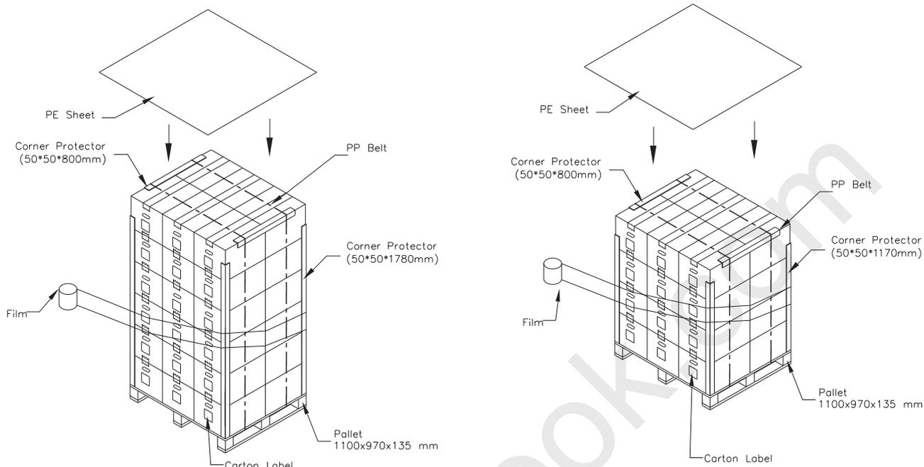
Figure. 9-2 Packing method
