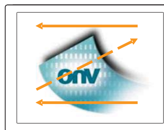
Fig. 2 Reverse scan (Pin19, REVERSE = High)
