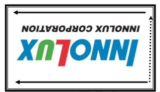
Fig. 1 Normal scan ( pin 4, LR/UD = High or NC )
