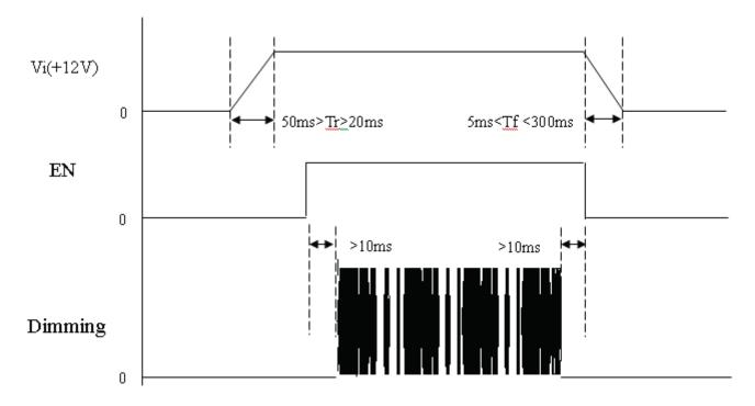
Note : While system is turned ON or OFF, the power sequences must follow as below descriptions Turn ON sequence:  $Vi(+12V) \rightarrow EN \rightarrow Dimming$ Turn OFF sequence: Dimming  $\rightarrow EN \rightarrow Vi(+12V)$
