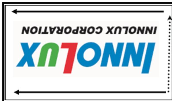
Fig. 2 Reverse scan ( pin 4, LR/UD = Low )
