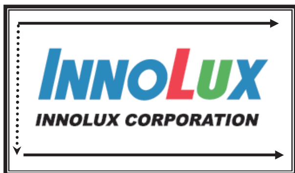
Fig. 1 Normal scan ( pin 4, LR/UD = High or NC )
