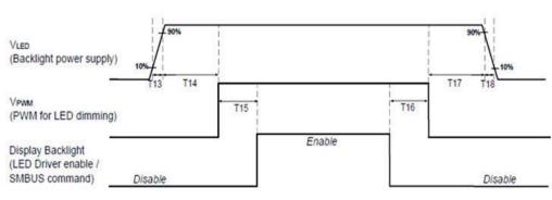
Note: When the adapter is hot plugged, the backlight power supply sequence is shown as below.
