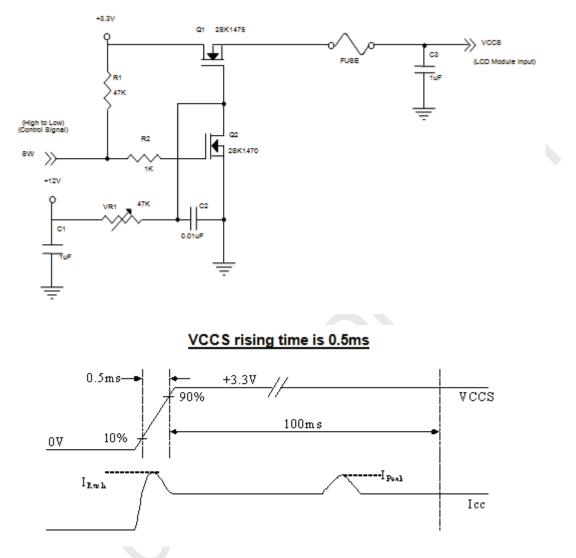
Note (3) The specified power supply current is under the conditions at VCCS = 3.3 V, Ta =  $25 \pm 2$  °C, DC Current and  $f_v = 60$  Hz, whereas a power dissipation check pattern below is displayed.
