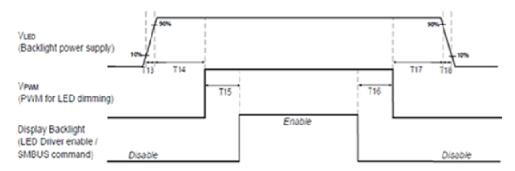
Note: When the adapter is hot plugged, the backlight power supply sequence is shown as below.
