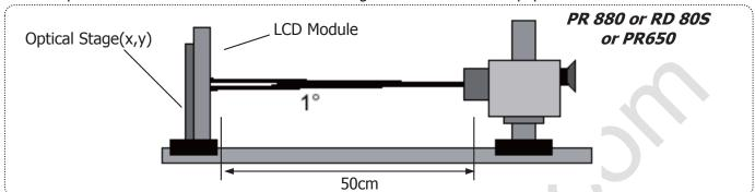
FIG.7 Optical Characteristic Measurement Equipment and Method
