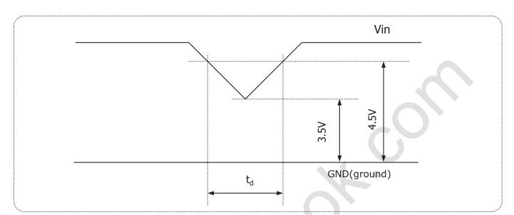
FIG.6 Power dip condition
