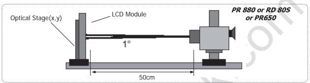
FIG.7 Optical Characteristic Measurement Equipment and Method
