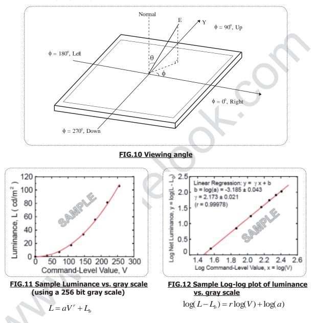
Here the Parameter a and  $\gamma$  relate the signal level V to the luminance L. The GAMMA we calculate from the log-log representation (FIG.11)
