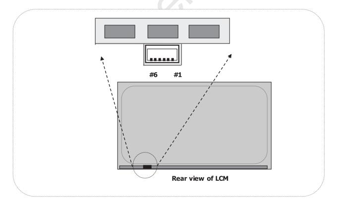
FIG.3-2 Backlight Connector View
