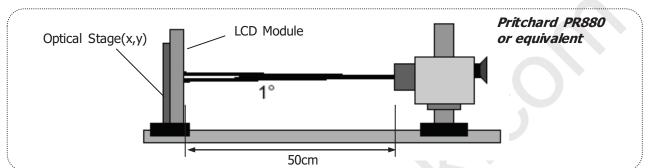
FIG.4-1 Optical Characteristic Measurement Equipment And Method
