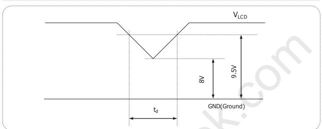
FIG.3-3 Power Dip Condition
