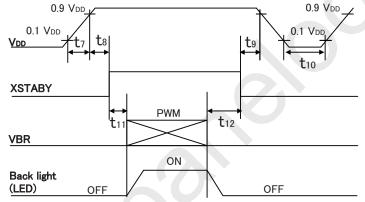
$20us \le t7 \le 10ms$   $0ms \le t8 \le$   $0ms \le t9 \le$   $1ms \le t10 \le$   $300ms \le t11 \le$   $300ms \le t12 \le$
