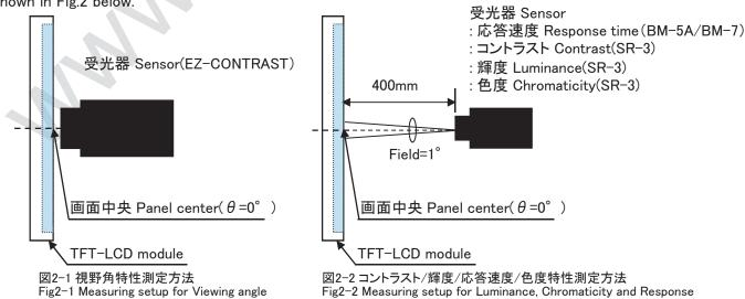
Fig2-2 Measuring setup for Luminance, Chromaticity and Response
