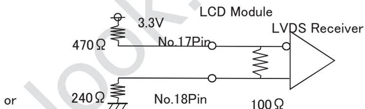
Recommended input (17pin, 18pin at 6bit)
