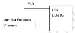
Note (2) For better LED light bar driving quality, it is recommended to utilize the adaptive boost converter with current balancing function to drive LED light-bar.
