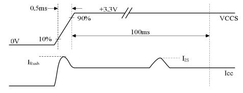
Note (3) The specified power supply current is under the conditions at VCCS = 3.3 V, Ta =  $25 \pm 2$  °C, DC Current and  $f_v$  = 60 Hz, whereas a specified power dissipation check pattern is displayed
