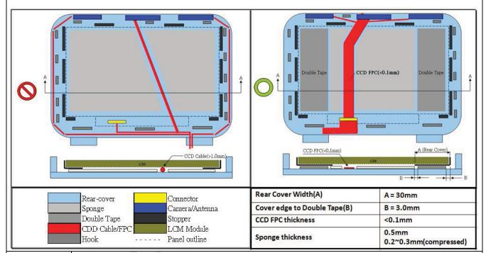
If the antenna cable or Web Cam wire must overlap with the panel outline, both sides of the antenna cable or Web Cam wire must have a sponge(Sponge material can not contain NH3) and sponge require higher antenna cable or Web Cam wire.( Antenna cable or Web Cam wire should not overlap with TCON,COF/FPC,Driver IC)
