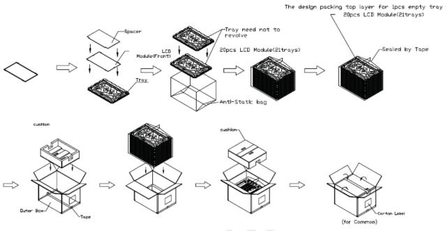
Figure. 7-2 Packing method
