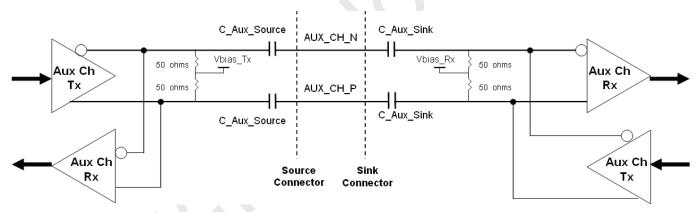
(3) Recommended Main Link Channel topology is as below and the Main Link AC Coupling Capacitor (C\_ML\_Source) should be placed on the source device.
