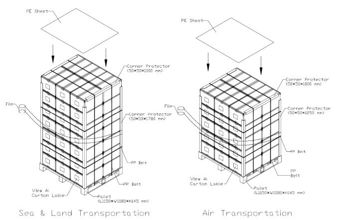
Figure. 7-3 Packing method
