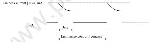
Duty:At the maximum luminance control 100% to at the minimum luminance control 1%. Luminance control frequency: 255 Hz (typ.)
