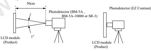
Note3: See "**4.11.2 Definition of contrast ratio**". Note4: See "**4.11.3 Definition of luminance uniformity**". Note5: These coordinates are found on CIE 1931 chromaticity diagram. Note6: Product surface temperature: TopF = (35)°C Note7: See "**4.11.4 Definition of response times**". Note8: See "**4.11.5 Definition of viewing angles**".
