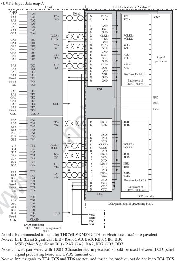
4.5.3 Connection between receiver and transmitter for LVDS (1) LVDS Input data map A
