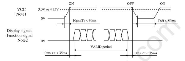
Note1: If there is a voltage variation (voltage drop) at the rising edge of VCC below 3.0V in "VCC = 3.3V'' or 4.75V in "VCC = 5.0V'', there is a possibility that a product does not work due to a protection circuit.
