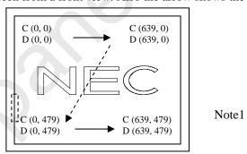
Figure 1. Normal scan (DPS: Low or Open)
