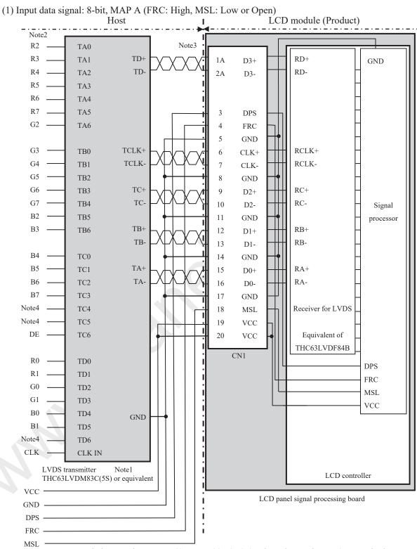
Note1: Recommended transmitter: THC63LVDM83C(5S) (THine Electronics Inc.) or equivalent
