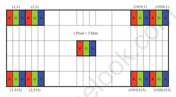
Figure 13. Display Position of Input Data (V-H)
