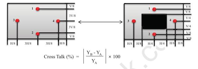
Figure 11. Cross Talk Modulation Test Description
