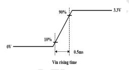
Figure 4. Inrush Measure Condition
