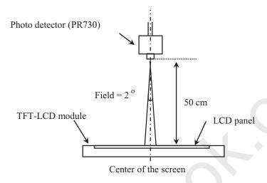
Optical characteristics measurement setup
