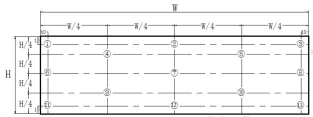
Figure 9. Uniformity Measurement Locations (13 points)
