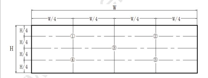
Figure 8. White Luminance and Uniformity Measurement Locations (5 points)
