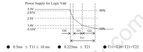
Figure 19. T11 timing requirements
