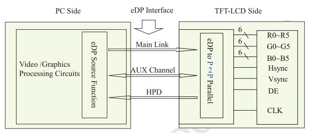
Figure 12. eDP Interface Architecture
