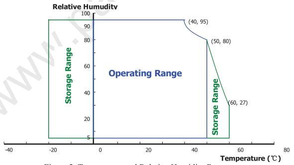
Figure 2. Temperature and Relative Humidity Range
