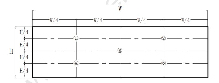
Figure 8. White Luminance and Uniformity Measurement Locations (5 points)
