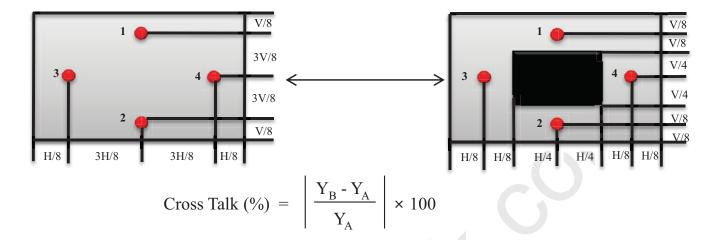
Figure 11. Cross Talk Modulation Test Description
