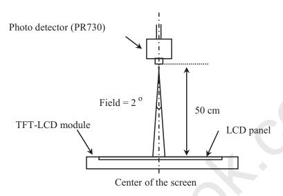
Optical characteristics measurement setup
