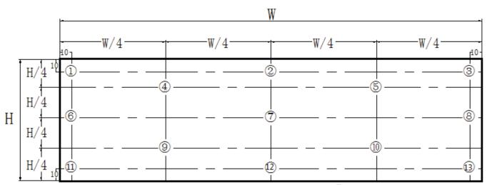
Figure 9. Uniformity Measurement Locations (13 points)
