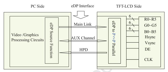
Figure 12. eDP Interface Architecture
