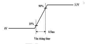
Figure 4. Inrush Measure Condition
