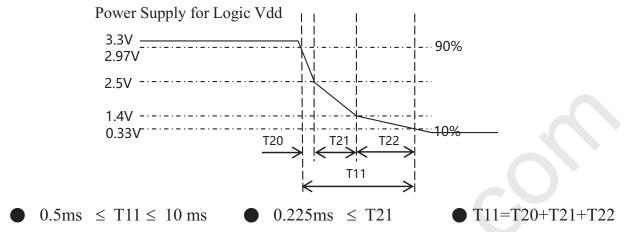
Figure 19. T11 timing requirements
