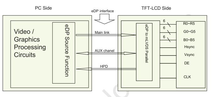
Note. Transmitter : Parade DP501 or equivalent. Transmitter is not contained in Module.
