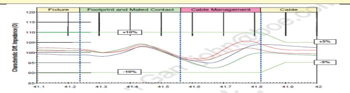
Differential Impedance Profile Measurement Data Example
