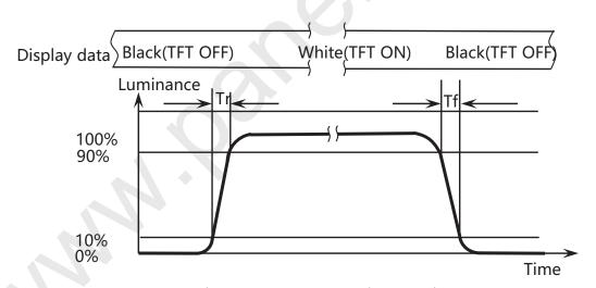
Figure 10. Response Time Testing
