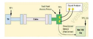
Measured TP3 on LCM connector.
