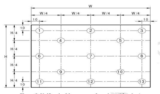
Figure 9. Uniformity Measurement Locations (13 points)
