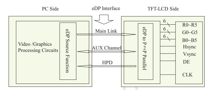
Figure 12. eDP Interface Architecture
