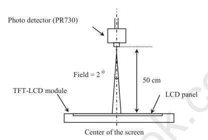
Optical characteristics measurement setup
