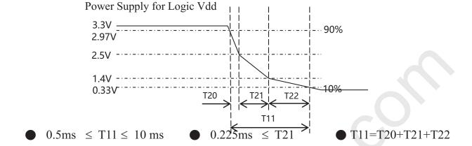
Figure 19. T11 timing requirements
