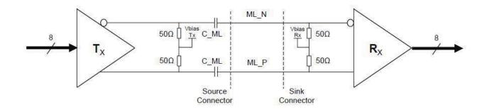
Figure 14. Main link differential pair
