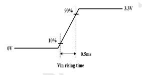
Figure 4. Inrush Measure Condition
