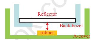
If sponge within the reflector area is necessary, we suggest that the gap b etween reflector and sponge is more than 0.5mm
