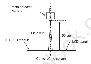
Optical characteristics measurement setup
