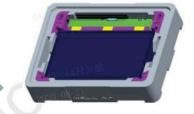
Put 1pcs Panel on the EPE Pad . Put one 2t EPE pad ... , totally 16 pcs Panel 、 16 pcs 2t EPE pads in one groove of box.
