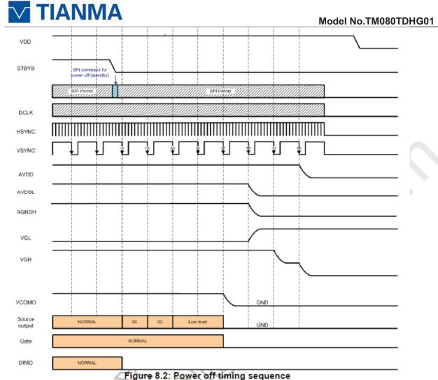
Note: Low level=3FH, when NBW=L (Normally white) Low level=00H, when NBW=H (Normally black)
