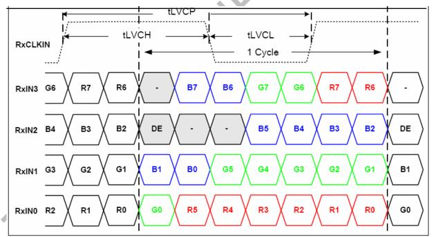
Figure 2.1.2 Input signal data mapping
