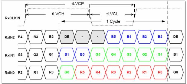
Note2: LVDS 6-bit data mapping when SEL68=L/NC as follows:
