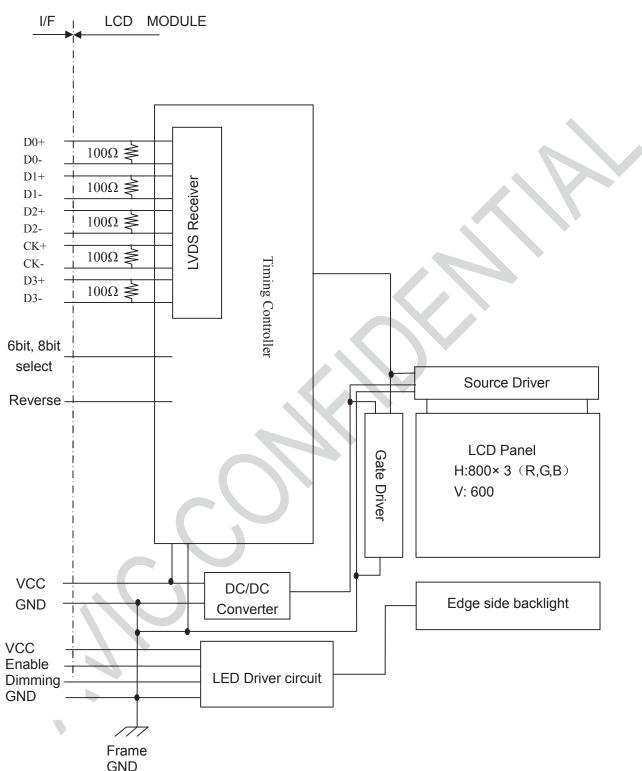
Note1: System ground (GND), Frame ground in the product should be connected together in customer equipment.
