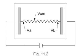
As shown in Fig. 11.2, applying voltage meter to measure Va, Vb and Vxm, where Va is the maximum voltage in the active area; Vb is the minimum voltage in the active area; Vxm is the measured voltage of point x selected by random. Afterwards, the linearity can be calculated by following equation:
