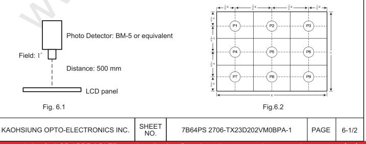
Note 3: The Contrast Ratio is measured from the center point of the panel, P5, and defined as the following equation:
