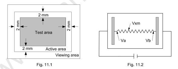
As shown in Fig. 11.2, applying voltage meter to measure Va, Vb and Vxm, where Va is the maximum voltage in the active area; Vb is the minimum voltage in the active area; Vxm is the measured voltage of point x selected by random. Afterwards, the linearity can be calculated by following equation:
