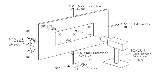
Figure 2. White Luminance and Uniformity Measurement Locations (9 points)
